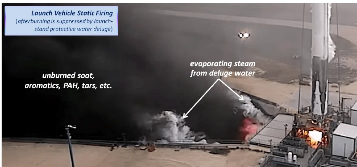
Figure 4. Exhaust from static-firing of full launch vehicle. The test-stand deluge water injected below the engine nozzles prevents damage to the test-stand by the hot plume during static firing, but the deluge water also quenches after-burning of the soot, aromatics, PAH, tars, etc. created by the gas generator and film coolant flows. The residual is present as the black cloud (PM2.5, PAH, aromatics, etc., left), about half way through the test-stand firing sequence for this vehicle. Compare this with the deposition of these effluents shown in Figure 5 (upper right) of the high-altitude afterburning shutdown sequence. [ref. C]
